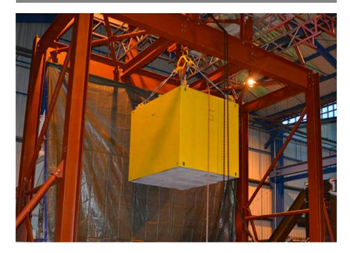
Initivo were commissioned to carry out specialist testing for the Nuclear industry. The project involved dropping an 18 tonne flask from 5 metres and was carried out at our indoor laboratory.
