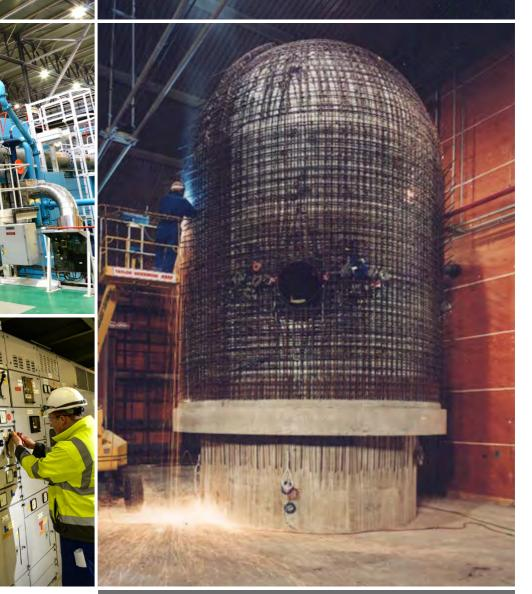
1/10th scale model of the Sizewell B (the last nuclear power station to be constructed in the UK) secondary containment structure. Design validation testing carried out.
