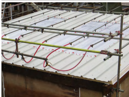
Standard roofing weathertightness test set up
